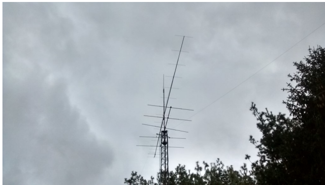
New Antenna (M2-5WL, 34 ft. long)
